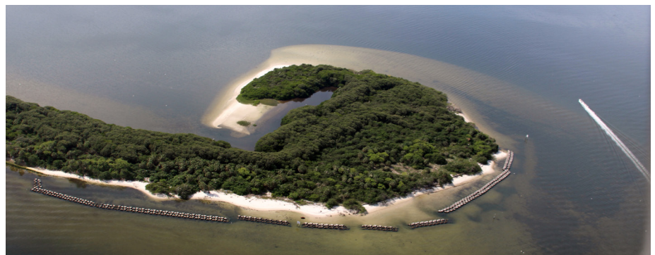
Breakwater reef protects Alafia Bank from destructive erosion. Photo: John Landon
